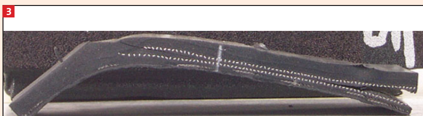
3 Peel Adhesion Test Specimen
